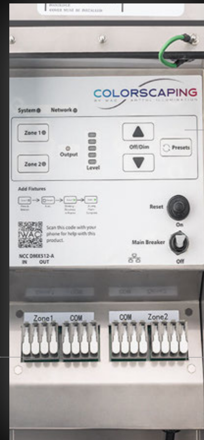
Control Colorscaping product using standard 2-conductor landscape wiring
